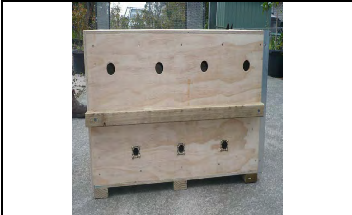
Figure 2: Side view of transport container showing upper and lower ventilation holes, handles stretching the whole length of the container, and three legs (K. Elliott, 2009).
