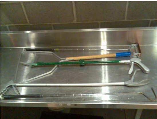
Pic 17: Selection of tools in order from top to bottom – Jiggers, hoop for hoop bag, two forms of grippers (food tongs, if padded correctly they can also be used as a snake grip) and snake hook.
