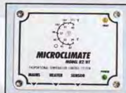
DL2 THERMOSTAT 101mm x 78mm x 41mm Microprocessor based (with alarms) pulse proportional thermostat for controlling up to 600 watts of NON LIGHT emitting heat source 04.DL2
