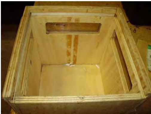
Left: Box interior. It can be clearly seen where the perch is going to be put above ventilation windows. The interior of the box is smooth and will be lined with fine gauze to dampen light and sound. Image, K. Jones.-2008
