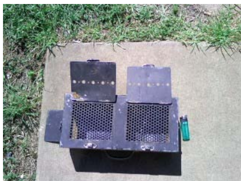
Aluminium metal twin cage 330mm x 170mm x 135mm. Lined with foam.
